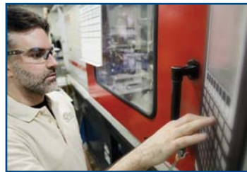
Greene, Tweed's most popular engineering thermoplastic was injection-molded Arlon 1000. Featuring lightweight strength, broad chemical resistance, and a wide operating temperature range, Arlon was utilized in every market. Common applications included back-up rings, seal assemblies, and electrical connectors.
