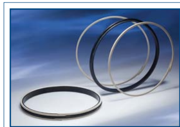
The wide base “T” geometry of the G-T Ring eliminated the problems of seal roll and spiral failure common found in O-rings.
