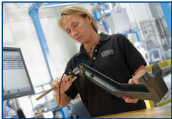
Xycomp thermoplastic composite was developed as a metal alternative. Up to 60% lighter than metals, it helped lower aircraft weight, reducing fuel burn and emissions. It also featured exceptional impact and fatigue resistance for extended service life.
