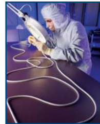
Extensis molding enabled the production of large seals for FPD (flat panel display) manufacture.
