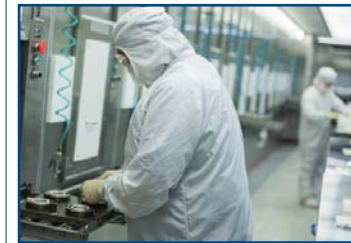
A class 100/1000 cleanroom was established in Kulpsville, PA in 1994. Designed for manufacturing semiconductor seals, it was the first of its kind in the United States.
