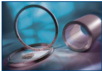
Greene, Tweed's most popular engineering thermoplastic was injection-molded Arlon 1000. Featuring lightweight strength, broad chemical resistance, and a wide operating temperature range, Arlon was utilized in every market. Common applications included back-up rings, seal assemblies, and electrical connectors.
