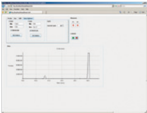
netMASsoft - a Java application for RGA operation directly from within your web browser.
