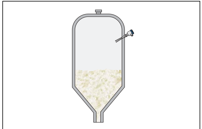
Fig. 1: Level detection in a silo storing plastic granules
